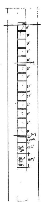
267' of 4" Black TtC pipe. 280' of #8 Sub Cable Suction @ 270.85' Runsfalled 1" + 3/4" Sounding tube 3005300 grundfor wetend 30 HP 460 V 3 Ph motor FLA 39.5 mLA45.2 LRA 284
